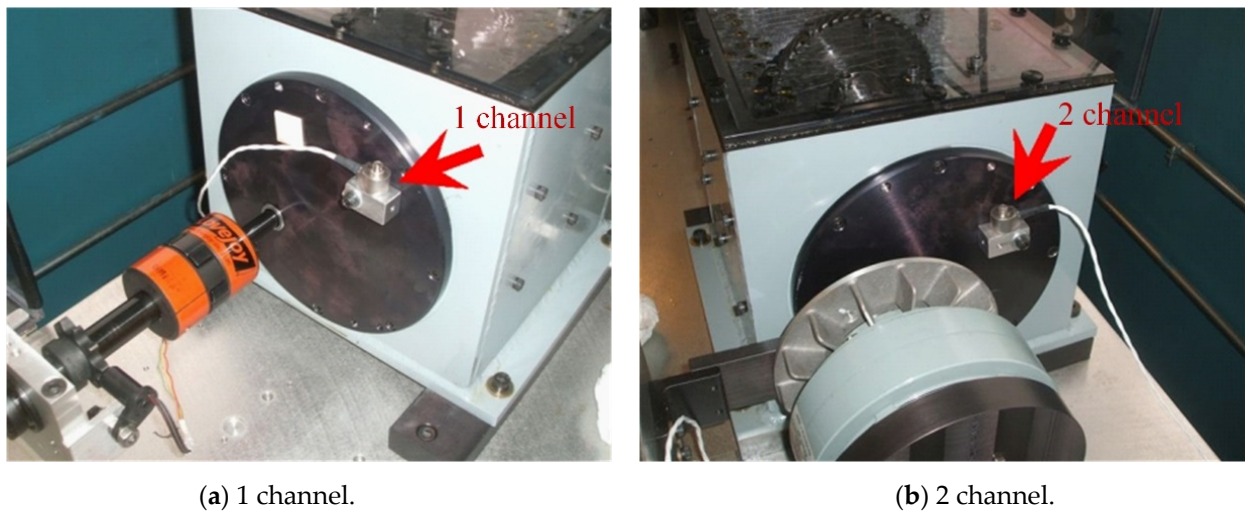
Figure 9. Accelerometers installation location.
