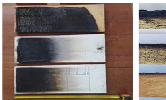
Fig. 2: Surface flame spread and cross-section respectively
