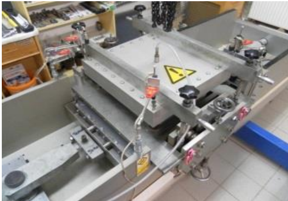
Figure 1.9: DS500 large-frame shear box device (Geotechnical Institute, TU Bergakademie Freiberg, Germany)
