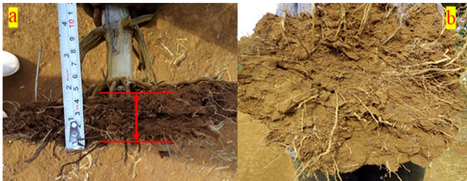
Plate 1. Mechanized tillage-induced compaction of the soil-root environment in Northrift, Kenya, (a) Maize rooting depth restricted to 4 cm (b) Impaired maize rooting penetration.
