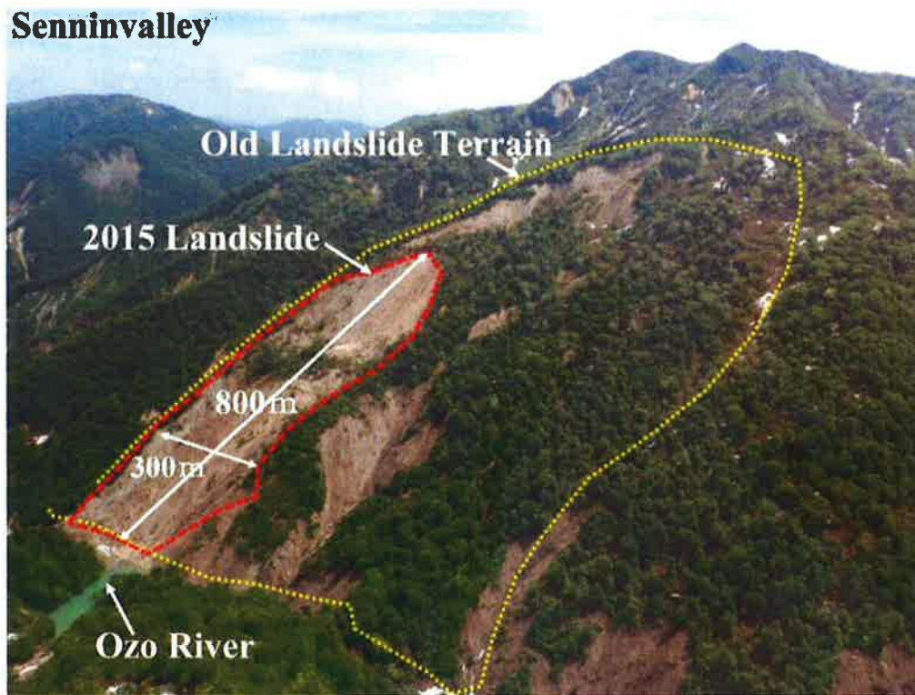
Figure 2 : 2015 Landslide overview showing the maximum horizontal length and width of the landslide (photo credit: Ishikawa Forest Management Office, 2016).
