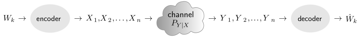
Figure 2.2: A discrete memoryless channel changes input symbol X_i = x_i to symbol Y_i = y_i with transition probability P_{Y|X}(y_i|x_i) .
