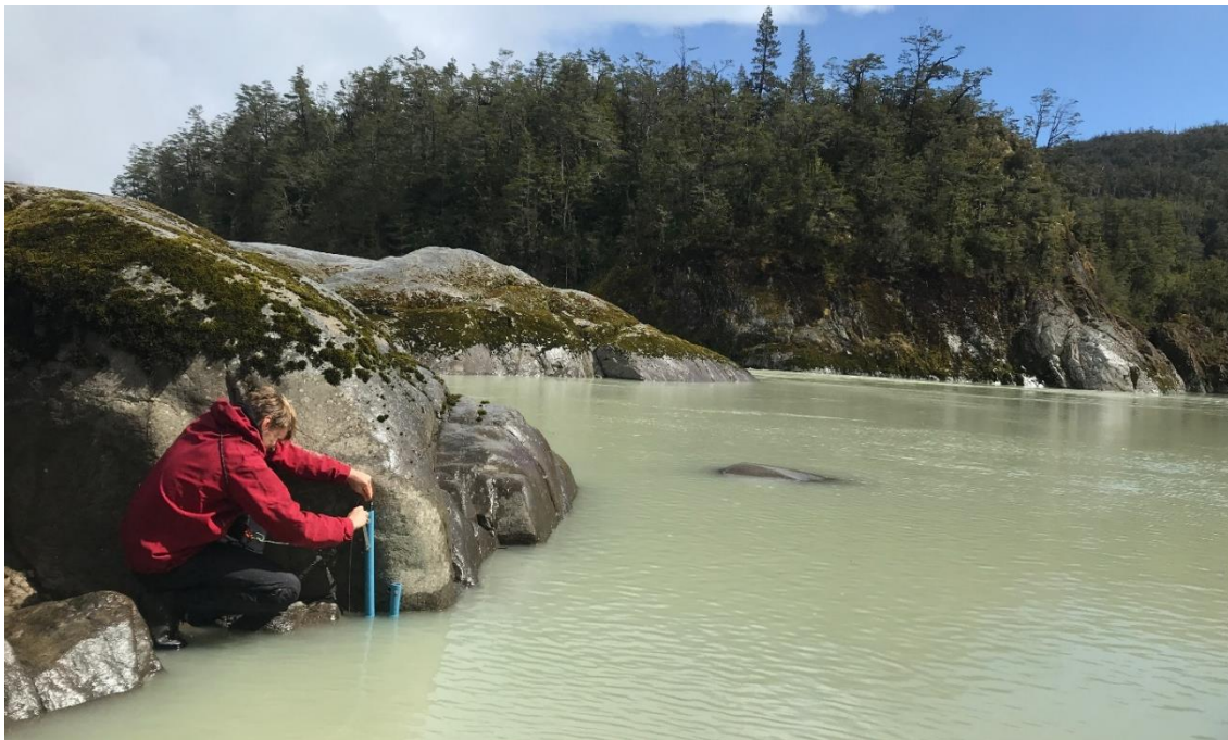
Figure 3.2: Location of the HOBO pressure transducer in a backwater pool (photo: Jemma Wadham).
