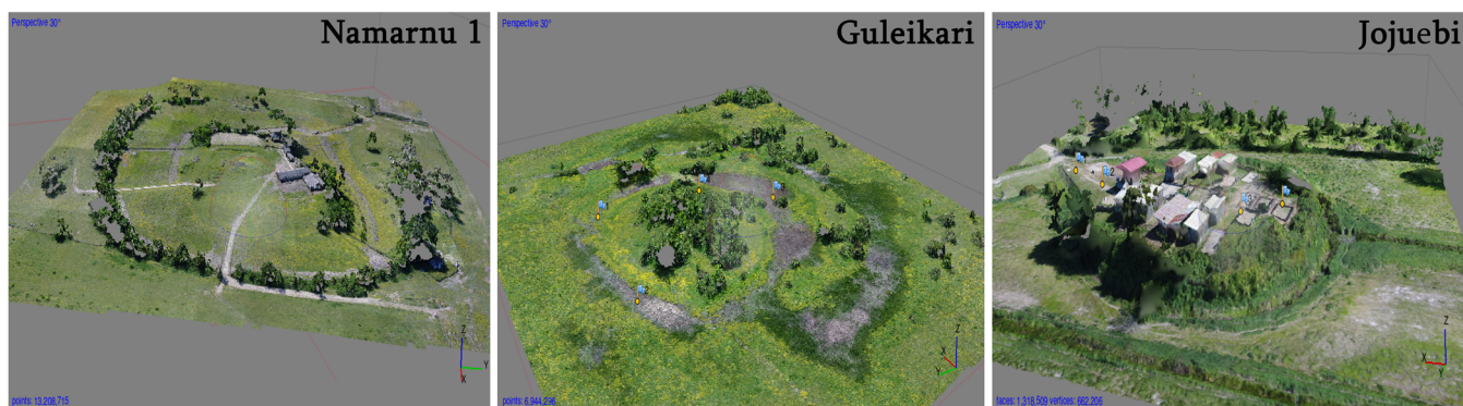
FIGURE 7 Structure-from-Motion three-dimensional model of the mound and surrounding area based on the aerial images (cf. Figure 4), processed with Agisoft Photoscan.
