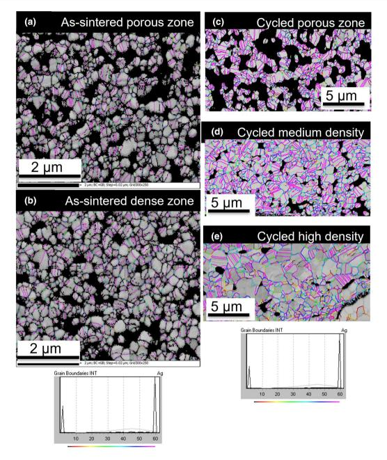
**Fig. 14** EBSD grain boundary maps of the (a) high-porosity and (b) high-density zones in the as-sintered sample, and (c) high-porosity and (d) intermediate-density and (e) high-density zones within the
