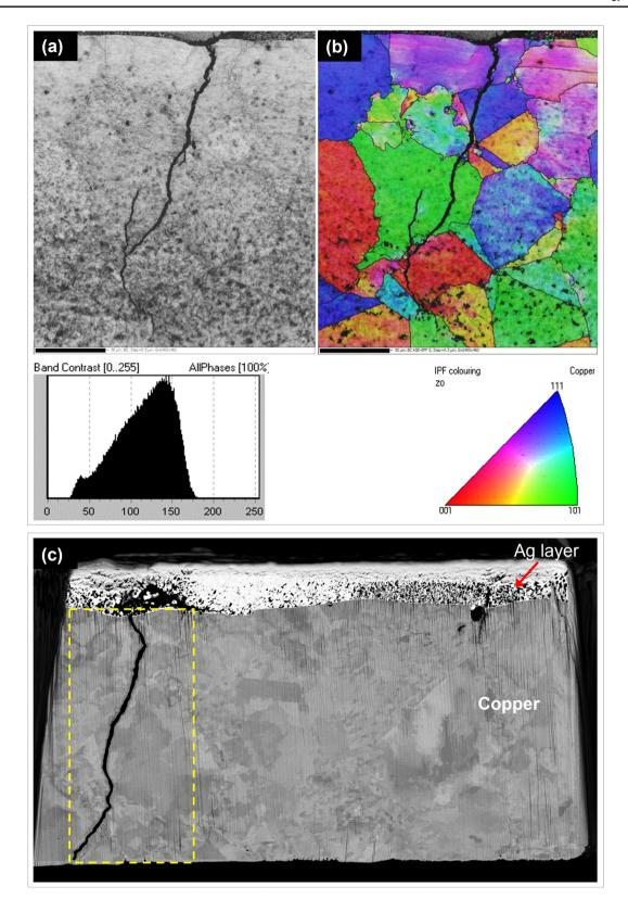
Fig. 19 Enlarged view of the crack labelled (I) in Fig. 18: (a) band contrast and (b) inverse pole figure (IPF) map in the Z viewing direction; (c) corresponding slice from reconstructed 3D FIB serial sectioning dataset.
