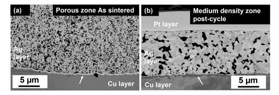
Fig. 5 Backscatter images showing the interface between the Ag sintered layer and the copper substrate for (a) a porous zone of the as-sintered specimen, and (b) the medium density zone of the cycled specimen.
