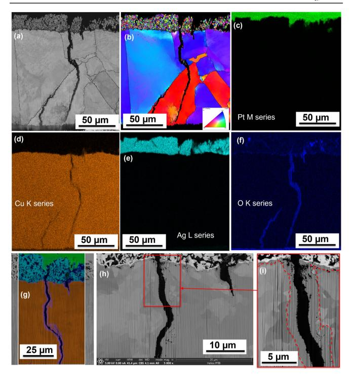
**Fig. 7** Spectral analysis of Ag-Cu interface and cracks. (a) EBSD band contrast image and (b) corresponding EBSD IPF representation of the selected region, step size  $0.2 \mu m$ . (c–f) EDS images showing
