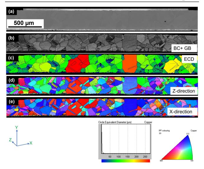
Fig. 17 (a) Backscatter image and (b–e) corresponding EBSD images for the as-sintered sample obtained using a step size of  $0.5 \mu m$ , (b) equivalent circle diameter (ECD) representation, (c, d) inverse pole figure (IPF) maps in the Z and X viewing directions, respectively.
