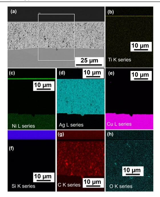
Fig. 6 (a) Electron backscatter image of the as-sintered bond showing the region selected for energy dispersive x-ray spectral (EDS) analysis. (b-h) Corresponding EDS images showing the spatial distributions of Ti, Ni, Ag, Cu, Si, C and O, respectively.
