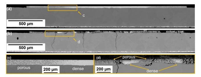
Fig. 4 Backscattered electron images of as-sintered (a, c) and cycled (b, d) samples showing regions of differing porosity.
