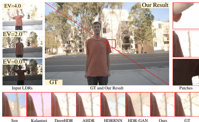
Figure 1: Three LDR images with different exposures are located on the left side. The image in the middle is our result and ground-truth (GT). EV denotes exposure value, which is determined by the exposure time, ISO and f-number.
