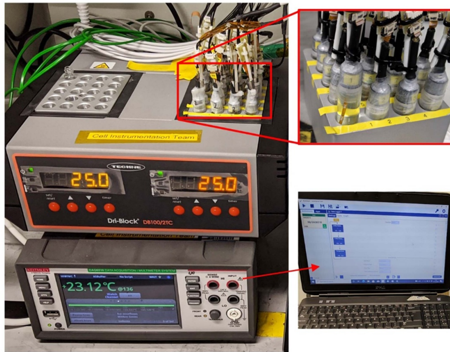
Figure 1. Photograph of experimental setup and data logging apparatus (block heater top, DAQ unit bottom). Inset image shows vials filled with electrolyte and sealed.
