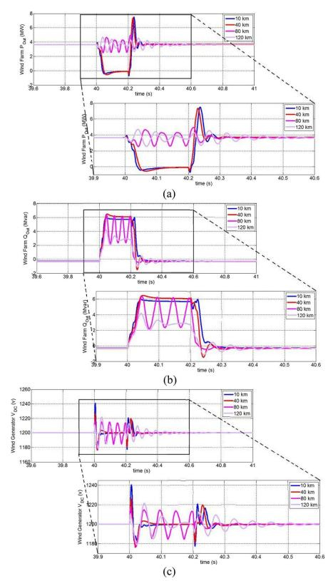
Fig. 9 Wind farm output parameters after single-phase short circuit fault. a Active power. b Reactive power. c DC link voltage
