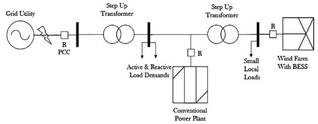
Fig. 6 Single-Line diagram of studied microgrid
