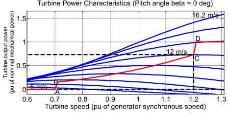
Fig. 8 Wind turbines power characteristic
