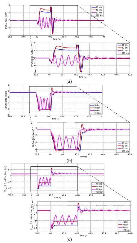
Fig. 10 25 kv Bus parameters after single-phase short circuit fault. a Active power. b Reactive power. c Conventional power plant output voltage
