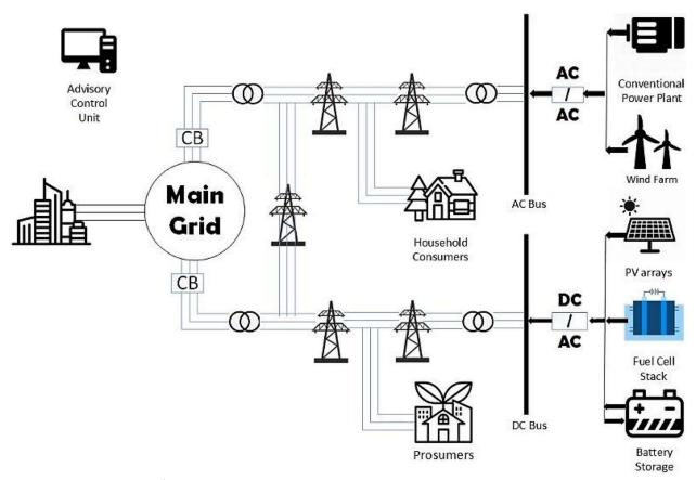
Fig. 2 Simultaneous operation of DC and AC units in a microgrid [64]
