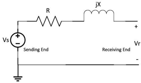
Fig. 3 Equivalent circuit of a short transmission line
