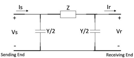
**Fig. 5** Equivalent circuit of a medium transmission line –  $\pi$  model
