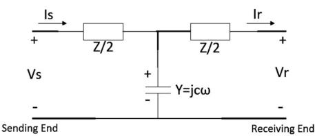
Fig. 4 Equivalent circuit of a medium transmission line – T model
