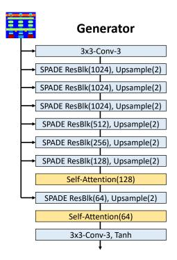
FIGURE 6.3: **The new generator.** Sketch of SPADE generator architecture after adding the self-attention module. It contains a sequence of SPADE residual blocks with upsampling layers. The last SPADE layer is between two Self-attention layers. The term 3x3-*Conv*-3 means a 3-by-3 convolutional layer with three convolutional filters, and *SPADE ResBlk* is the SPADE residual block. We made the network deterministic by starting with a downsampled segmentation map instead of random z.
