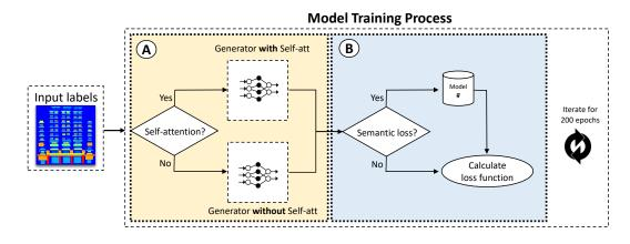
FIGURE 6.2: The training process. This image highlights the two contributions we made to the SPADE model targeting the synthetic image quality enhancement. (A) The self-attention mechanism and in (B) the semantic loss. Both can be turned on/off, and therefore we have four training possibilities: both off, which is the original SPADE model. Alternate on, and both on. That brings four different models. See Table 6.2 for the possibilities.
