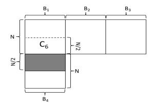
FIGURE 4.7: **Inner row conditioning.** How the condition of the first block of an inner row i > 1 is selected. The condition  $C_6$  is used to generate the top half part, in grey, of block  $B_4$  in this example.
