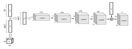
FIGURE 4.3: **Generator architecture.** Initially, the  $64 \times 64$  input patch is reshaped and then concatenated with the input noise vector *z*. Finally, before being processed by the last layer, the output of the penultimate layer is concatenated with the condition vector *S*.
