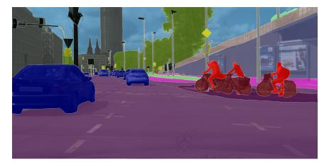
FIGURE 2.1: **Semantic Segmentation.** Image segmentation performs its task by assigning a label to each pixel in a source image. This example is taken from the Cityscapes dataset [27], one of the datasets we use in our work.
