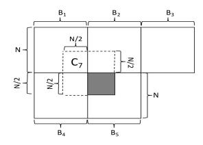
FIGURE 4.8: **Inner block in an inner row conditioning.** How the condition of the inner blocks in a inner row i > 1 is selected. To generate the top left part of block  $B_5$ , in grey, a corner condition is selected from the blocks  $B_1$ ,  $B_2$  and  $B_4$ .
