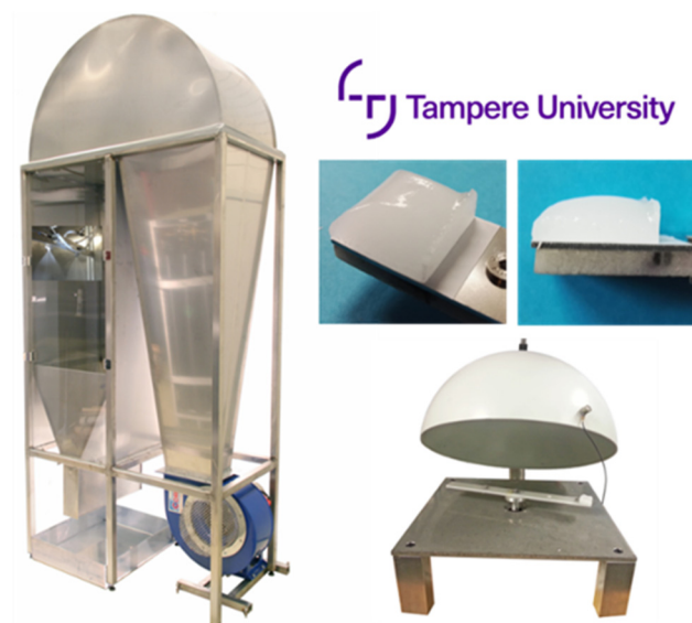
Figure 5. Icing wind tunnel (IWIT), centrifugal ice adhesion tester (CAT), and examples of mixed glaze ice accreted on test samples at Tampere University (TAU), Finland.
