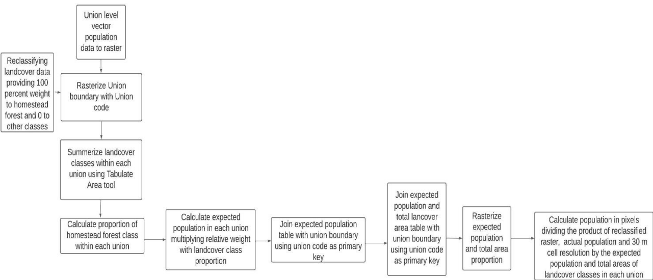
Figure 2.4 Workflow raster-based dasymetric mapping and population displacement.
