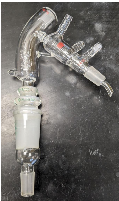
Figure 34: Vacuum jacketed, short path distillation head used for the purification of CBA n -1. Adapters installed to prevent overflow in the case of bumping.
