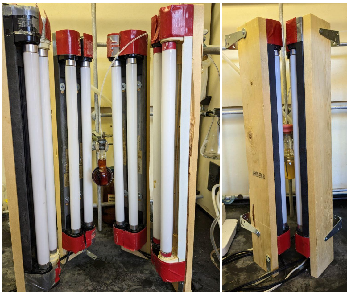
Figure 32: Simplified reaction apparatus for synthesis of CBAn-1 known as the Light Array for Photochemical Reactions Apparatus or LAPRA. Left: LAPRA in open position for easy access to mixture. Right: LAPRA in closed position.
