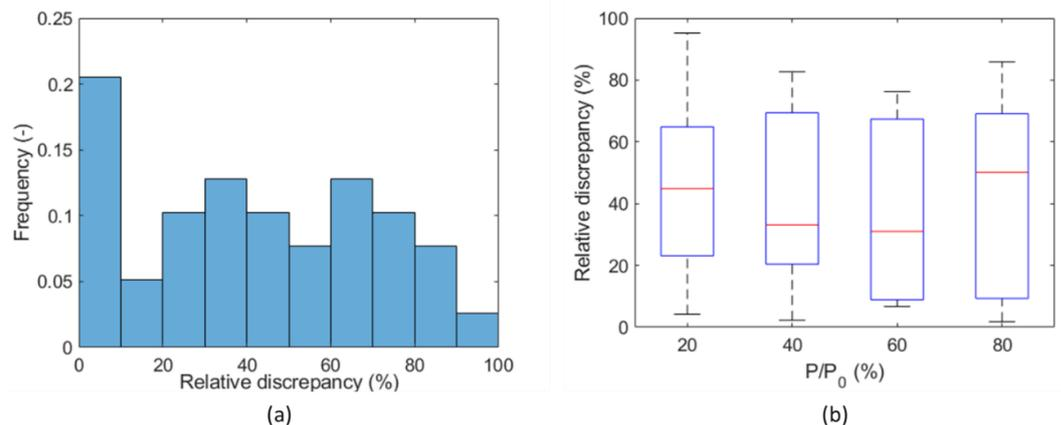
**Figure 14.** Uncertainty analysis exploring the reproducibility of the experiment: relative discrepancy on diffusion coefficient between Test a and Test b (Caprock1 and Caprock2) (a) for all partial pressure steps and (b) for each partial pressure step.
