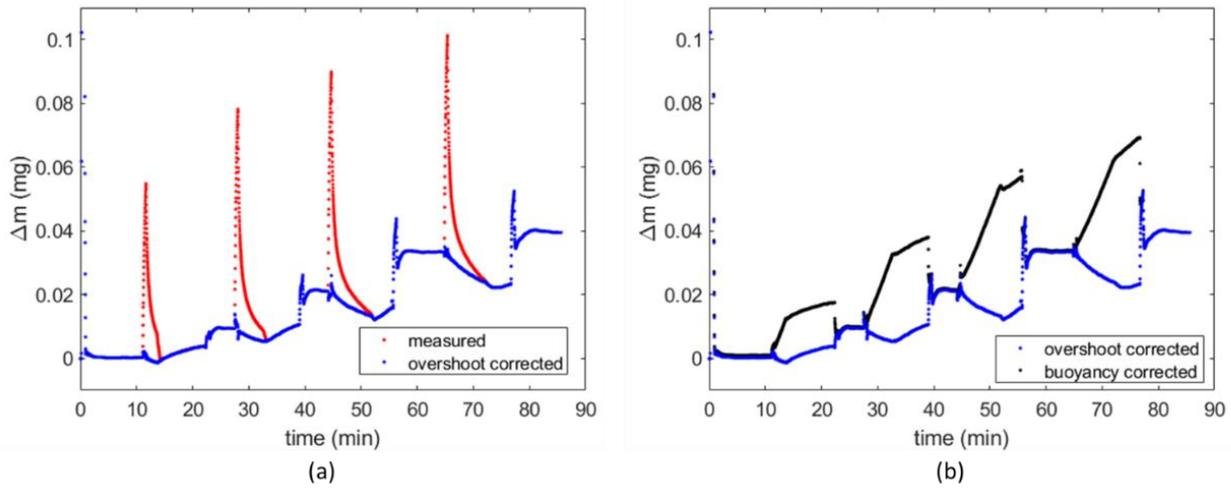
**Figure 7.** Measured mass variations in time and correction for (a) overshooting and (b) buoyancy (test FR4\_CH4\_a).
