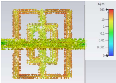
Fig. 12. Field images of surface current density, cut-slot structure with CN present, at 4.68, CN lines GHz.
