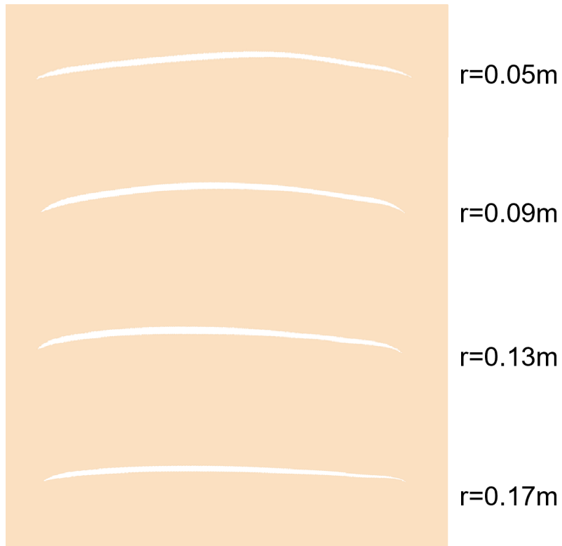
Fig. 11 Normalized airfoil sections at different radial stations after adjoint optimization. Three-bladed rotor.
