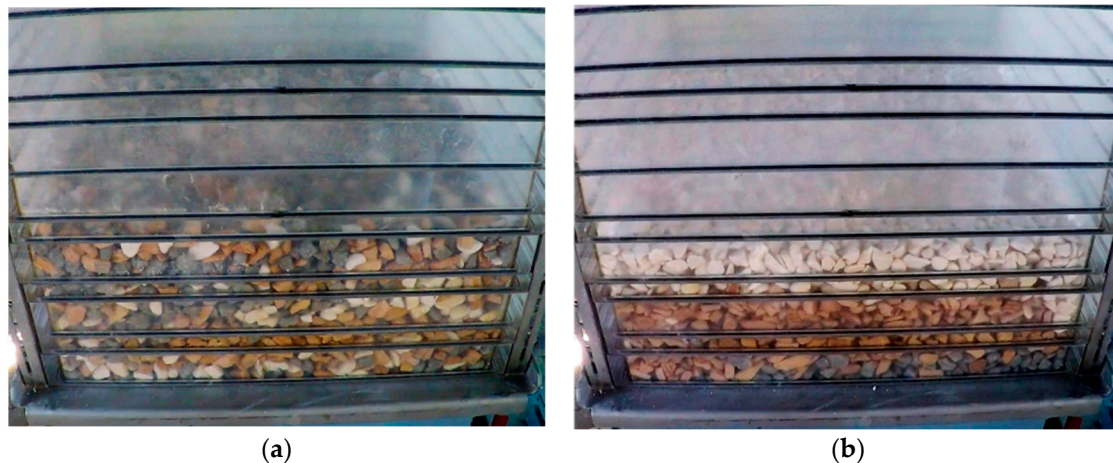
Figure 13. Snapshots of the separation of ternary mixture of gypsum (white), brick (reddish), and concrete (gray) captured by camera positioned at the upper diagonal of a pilot-scale dry jig. (a) Mixed state (before separation); (b) Segregate state (after separation).
