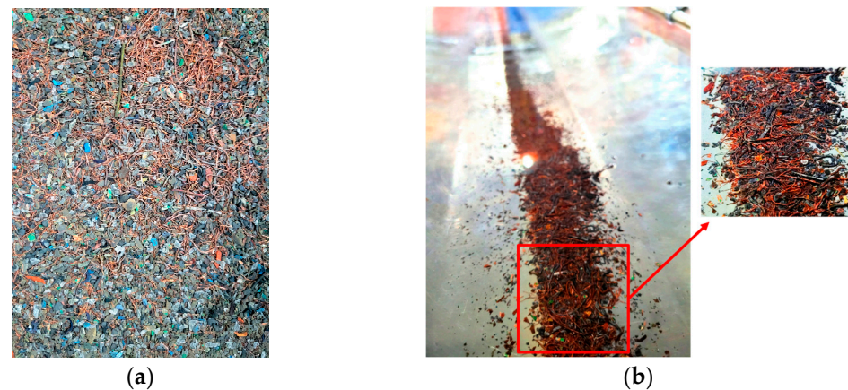
Figure 14. Separation of crushed PCBs ( -2 mm) in a Mozley table. (a) Initial mixture; (b) Metallic concentrate on the table surface.
