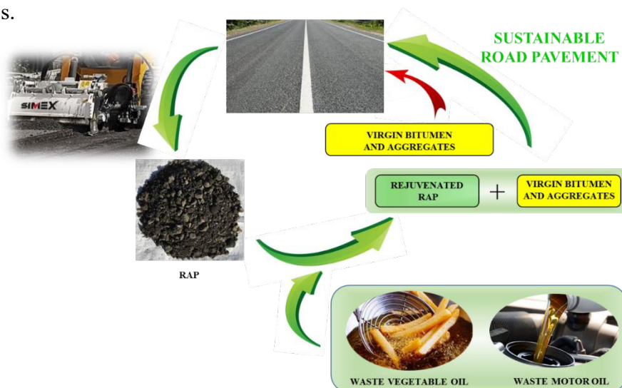
Figure 1. Schematic approach to realize a sustainable road pavement using RAP rejuvenated using waste oils.
