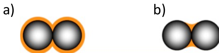
Figure 1.8 The coating distribution over aggregate can be (a) uniform coating or (b) between junctions of the spheres.
