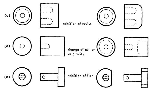
Addition of External Features to Reduce Difficulty of Sensing Orientation
