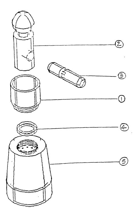
Exploded View for Shower Head Assembly Automatic Assembly
