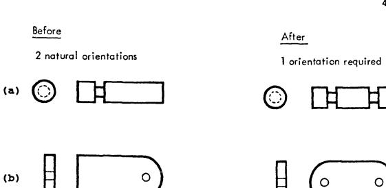
Use of symmetry to simplify parts orientation.
