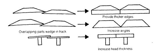
Shingling or Overlapping Can be Avoided by Providing Thicker Contact Edges, or Increased Angles, or Thicker Heads.
