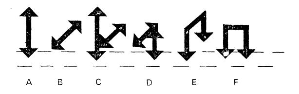
(a) Typical Standard Placement Device Motions
