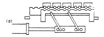
Walking Beam Transfer Mechanism
