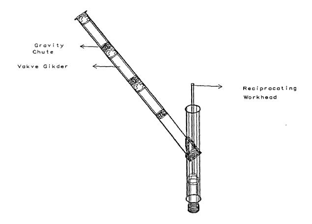
Part Placing Mechanism
