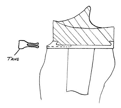
Side Loading Tibial Insert with Dovetail/Tang
