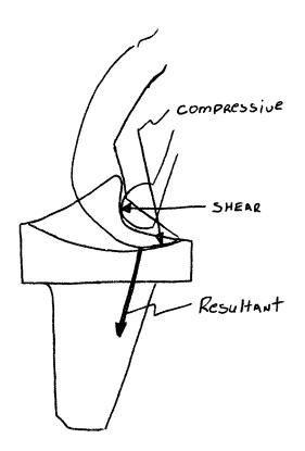
Resultant Force for Tibial Component of the Insall-Burstein
