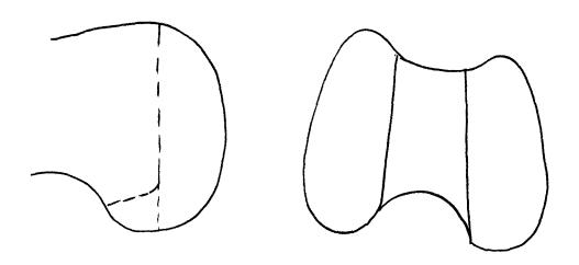
Distal Femur with Typical Resection for Femoral Housing
