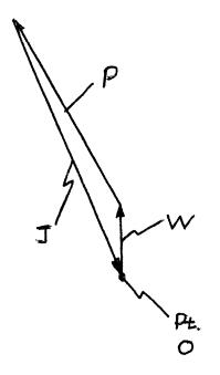
Graphical Determination of Joint Reaction Force
