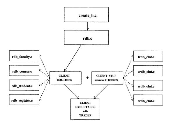
Figure 5.7: Production Process of the Trader using RPC
