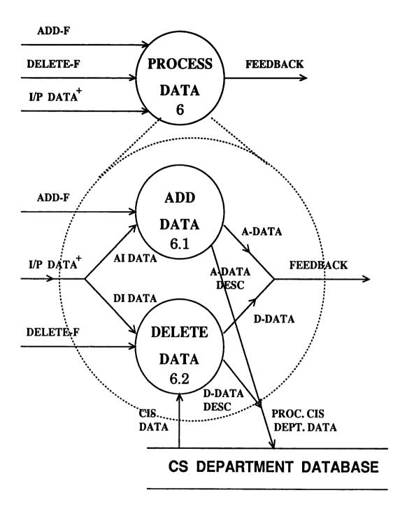
Figure 3.4: Level 2: PROCESS DATA
