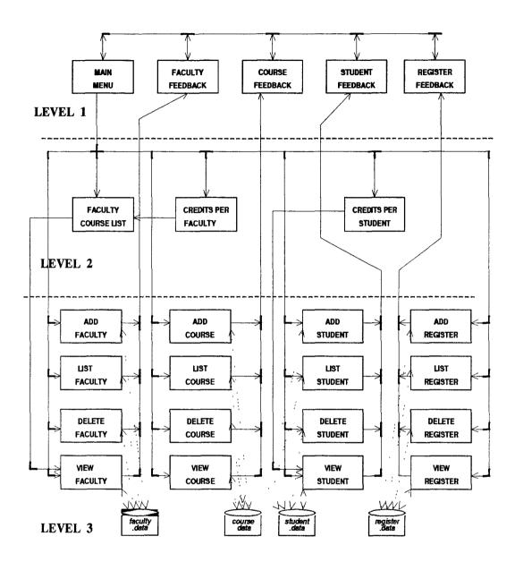
Figure 4.10: Communication between Building Blocks on a Conceptual Level
