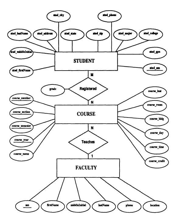
Figure 3.1: ER Diagram for CS Department DIS
