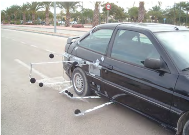
Fig. 13. Configuration used in the final A-CPX tests.
