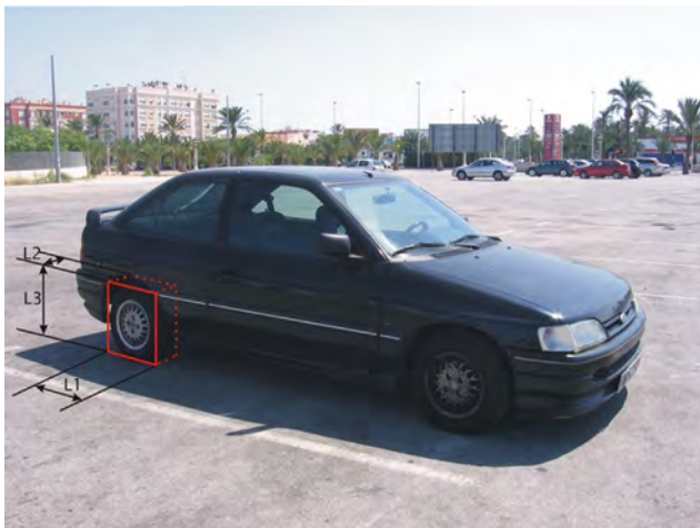
Fig. 1. Parallelepipedic reference surface defined for the A-CPX test.
