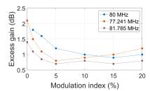
**Fig. 3.** Excess gain for the observed ML threshold, in dB, at different shifting frequencies  $f_s$  and electrical modulation indices  $\mu$ . Zero modulation index refers to a situation where the AOFS is driven by a single RF tone without AM, for which ML induction at  $f_s = 80$  MHz was not possible in our laser.
