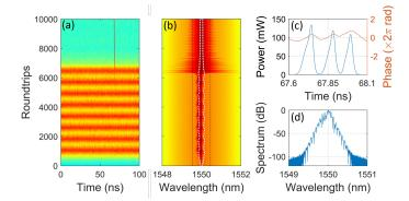
**Fig. 5.** Intensity (a) and spectral (b) maps of the self-starting ML regime induced by Kerr effect (see **Visualization 1**). (c) Pulse intensity and phase and (d) optical spectrum at the final recirculation. In (b), the dashed lines represent the filter's FWHM and the white dotted trace the frequencies where the filter is at threshold.
