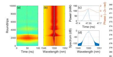
**Fig. 6.** Same as in Fig. 5 but with a loss of 16 dB and triggered by AM ( $\mu = 0.005$ ) during the first 5000 recirculations. The final pulse width is 58 ps (FWHM). See Visualization 2.
