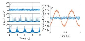
**Fig. 2.** Intensity of the CW regime of the FSF laser at (a)  $f_s =$ 80 MHz, (b)  $f_s = 81.785$  MHz ( $f_s \tau_c = 9$ ), and (c)  $f_s = 80$  MHz with AM modulation ( $\mu = 0.005$ ). (d) Intensity recorded after the AOFS when driven by a  $f_s = 80$  MHz tone (blue) and by the same tone with an additional AM modulation with  $\mu = 0.02$  and modulation frequency of 2 MHz (orange).
