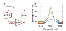
Fig. 1. (a) Scheme of a FSF laser. (b) Optical spectrum of the FSF laser in different regimes: blue, below threshold; orange, CW emission above threshold; green, self-starting ML emission; and magenta, AM-triggered ML emission.
