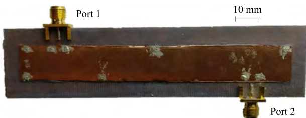
Fig. 12. Photograph of the final fabricated filter after the manufacturing process is completed.
