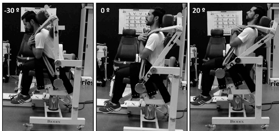
Figure 1. Participant performing a maximum effort of trunk flexion–extension in the isokinetic dynamometer with a ROM of 50^\circ ( -30^\circ trunk flexion; 0^\circ initial position; 20^\circ trunk hyperextension).
