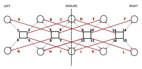
**Fig. 2.** The optode arrangement of the device. The squares represent the emitters, and the circles represent the detectors. The short channels are represented by black arrows with the numbers 1–16, while the long channels are represented by red arrows with the letters A–L. The montage was placed on the forehead, covering a part of the prefrontal cortex. (For interpretation of the references to color in this figure legend, the reader is referred to the web version of this article.)
