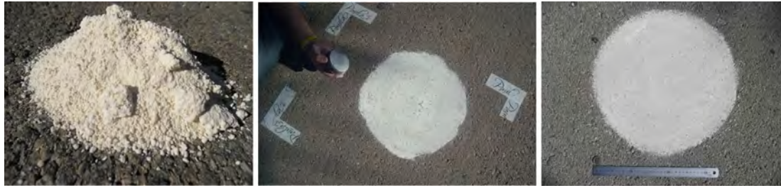
Fig. 4. Sand sample used for the MTD tests, test procedure and measurement point.
