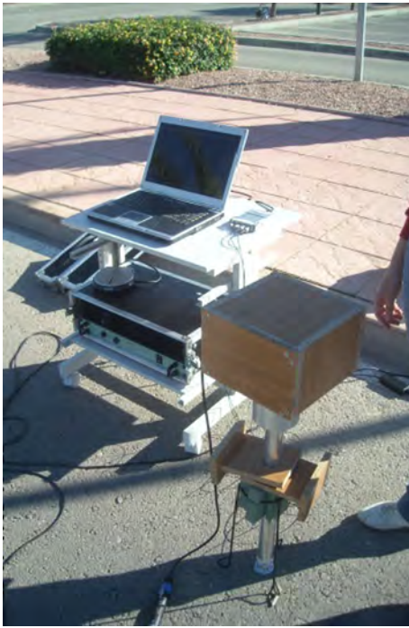
Fig. 3. Sound absorption coefficient measurements set-up.
