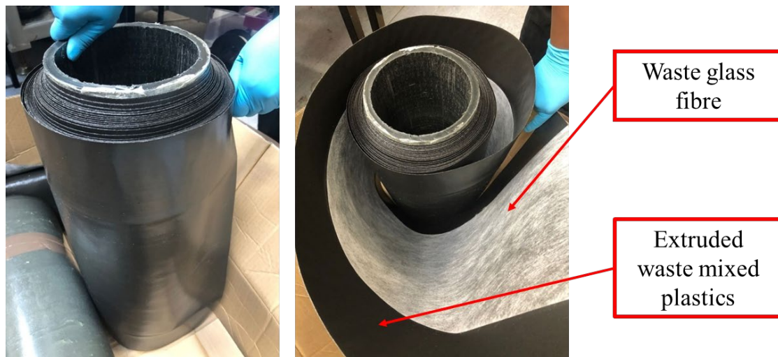
Figure 3: Manufactured roll (thermoplastic prepreg) of waste mixed plastic (wMP) coated waste glass fibre (wGF).
