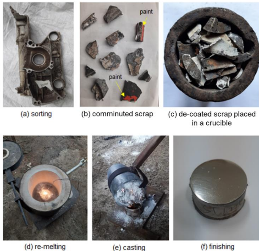
Figure. 1. The recycling process of the magnesium scrap in this research.
