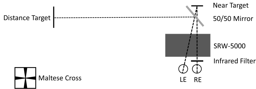
FIGURE 1 Schematic representation of the subject's right (RE) and left eye (LE) with target alignment. Both near (33 cm) and distance (4 m) targets were size-matched Maltese cross targets, each displayed in an internally illuminated light box. The subject viewed the distance target with the LE with the contact lens (CL) in place, via the 50/50 mirror. The near target was at 33 cm from the eye. Step changes in stimulus vergence were achieved by illuminating these targets in turn.
