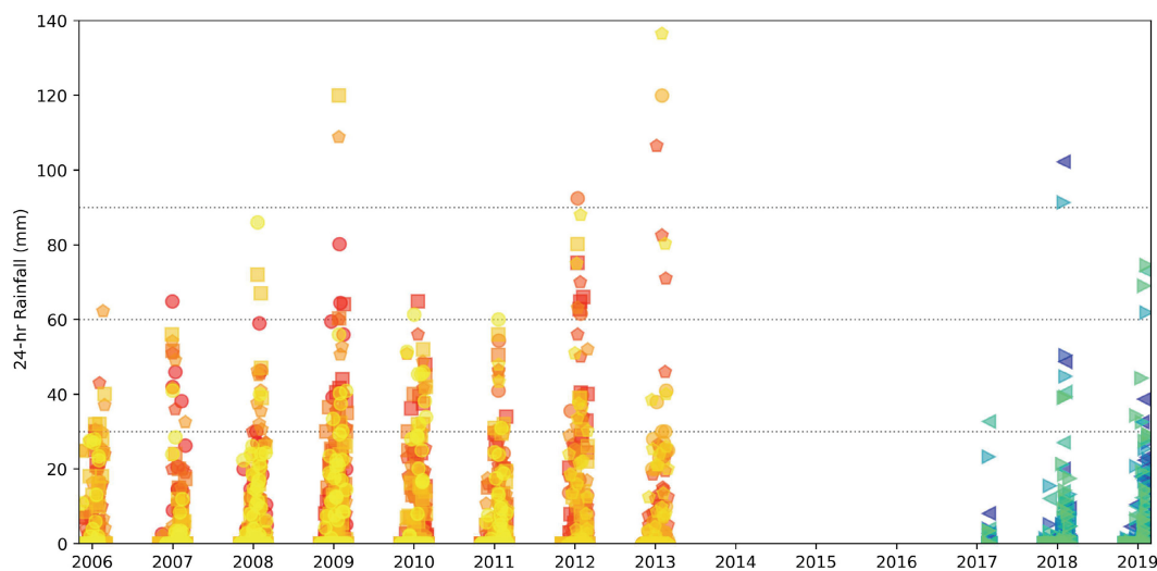
FIGURE 2 Precipitation 24-hour accumulation values for the 16 Dakar rain gauges used for verification. Data from the 10 manual rain gauges are shown from 2006 to 2013, with data from the six automatic rain gauges shown from 2017. Each rain gauge is shown by a different colour–shape combination. [Colour figure can be viewed at wileyonlinelibrary.com ]
