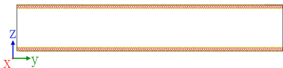
Fig. 1. Schematic illustration of the nano slit pore. The pore width equals to 86.6 Å with dimensions x and y of 24.6 and 595 Å.
