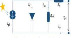
Figure.1.circuit equivalent panel solar [13]
