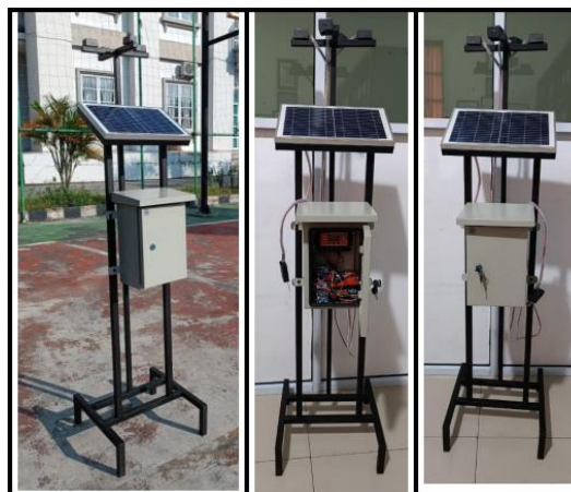
Figure 8. Display of a Fire Detector
