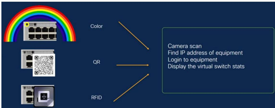
*Figure 12: Example Integration of Universal Status Light and Identifier*
