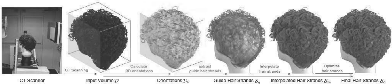
Fig. 2. Overview of our method. We use an industry CT scanner to obtain 3D density volumes. The first stage (Sec. 3.2) extracts reliable guide strands by estimating 3D hair orientation fields. The second stage (Sec. 3.3) refines the interpolated guide strands using the input density volume.
