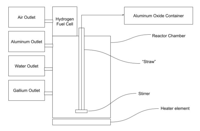
Claim 1: A reactor system for the controlled chemical reaction between aluminum and water in the presence of gallium, facilitating the generation of hydrogen gas and aluminum oxide, comprising:
