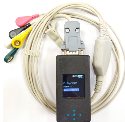
Figure 15. CAECG monitor developed with electrodes' cable.
