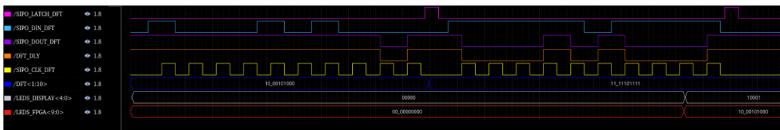
Figure 53. Reception of the sequence “1000101000” with no delay
