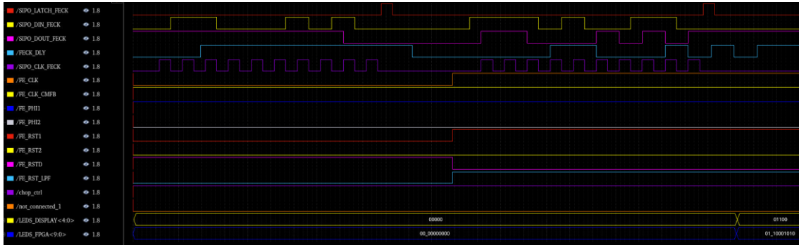
Figure 59. Reception of the sequence “0110001010” with 3 serial clock period delay (FECK SIPO)
