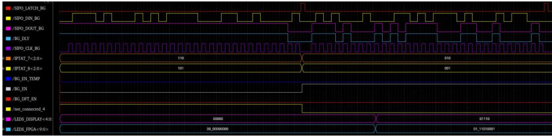
Figure 50. Reception of the sequence “0111010001” with no delay
