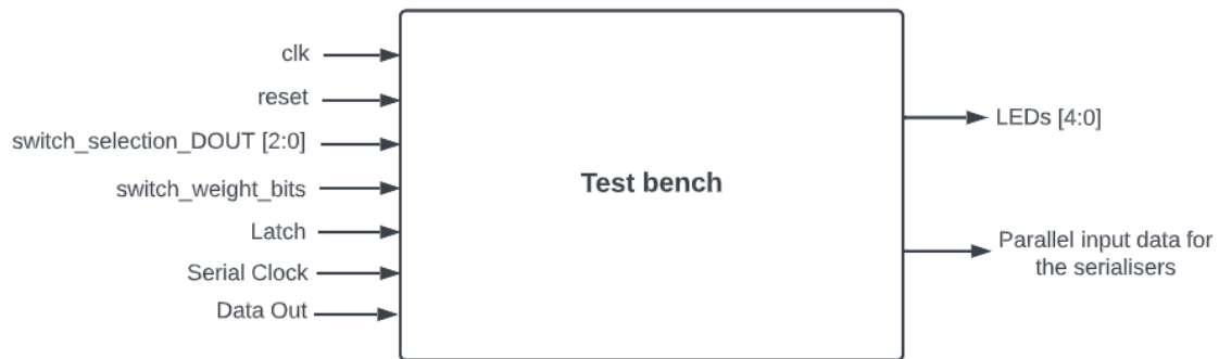
Figure 37. Block diagram of the SIPOs test bench
