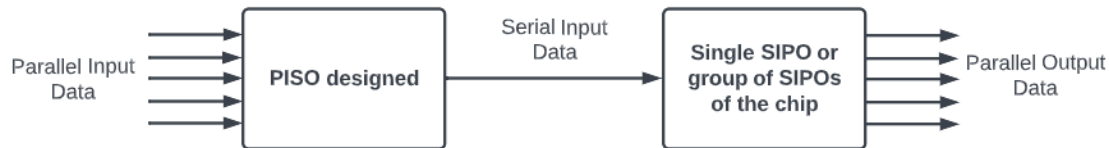
Figure 9. Block diagram of the circuit used to test the SIPOs of the chip
