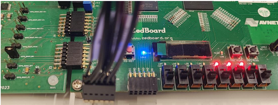
Figure 92. Reception of the data transmitted to the BG SIPO (MSB)
