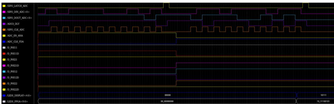
Figure 67. Reception of the sequence “1011100101” with 1 serial clock period delay (ADC SIPO block 0)
