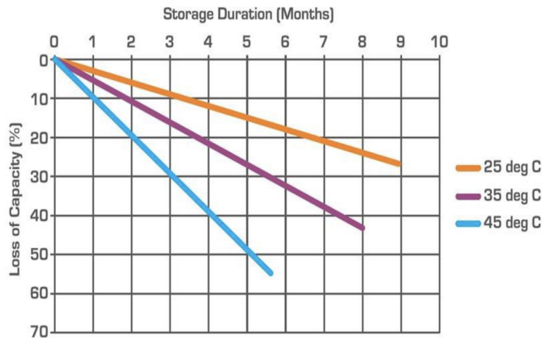
Figure 27: Temperature effect on self-discharge rate (Ansari, 2022).
