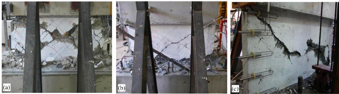
Figure 6. Diagonal tension (a) T1-S1, (b) T1-S2, (c) T1-N10-S1. Source: Terzioglu et al. (2018).
