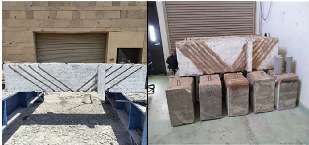
Figure 7: Tested specimens after retrofitting.
