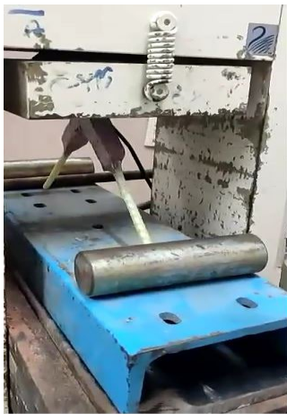
Figure 4: Testing of the internal GFRP stirrup joint.
