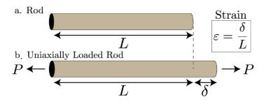
Figure 31: Strain mechanism.
