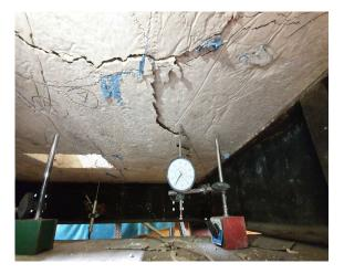
Figure 11: LVDT to measure slab deflections.
