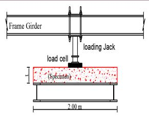
Figure 9: Illustration for the loading machine
