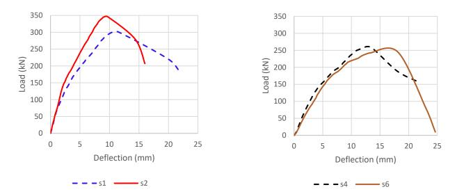
Figure 18: Load versus mid-span deflection for flat slab subjected to 4 and 6 strands for "control specimens", which without any openings, (S1 and S2).
