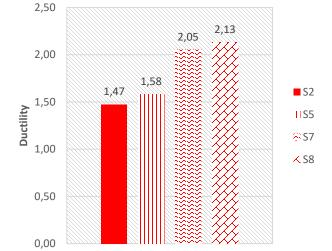
Figure 23: Ductility induced from 4 strands post-tensioned flat slab.
