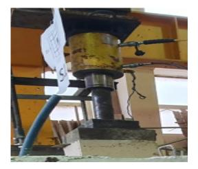
Figure 10: A metal plate between the jack of the loading machine and the concrete.
