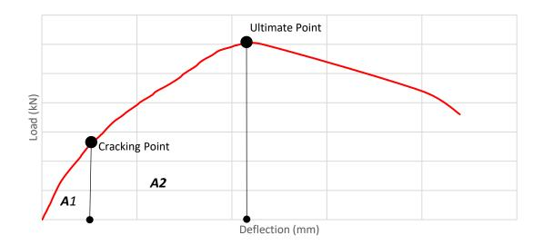
Figure 28: Indication for Calculating the Energy absorbed from Area under curve
