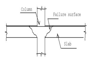
Figure 34: An illustration for Punching failure surfaces of tensioned flat slab.
