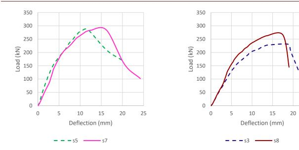
Figure 20: Load versus mid-span deflection for flat slab subjected to 6 strands specimens "specimens with openings either before or after Casting" (S5 and S7).
