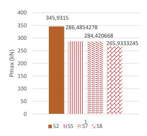
Figure 14: Load comparisons between control Specimen(S1) and specimens with openings subjected to 4 strands
