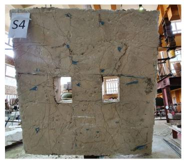
Figure 1: This slab shows us the form of punshing failure and cracks if there are two holes next to the column.
