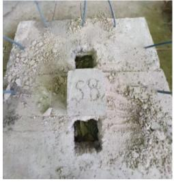
Figure 6: (S 8) After making the two holes and cutting the strand. Figure 7: A picture to illustrate the shape of the opening after
