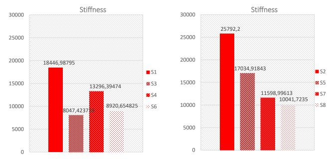
Figure 26: Stiffness induced from 4 strands post-tensioned flat slab. Figure 27: Stiffness induced from 6 strands post-tensioned flat slab.
