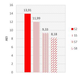
Figure 29: Energy Absorbed induced from 4 strands post-tensioned flat slab.
