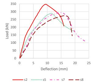
Figure 12: Load versus mid-span deflection for flat slab subjected to 4 strands, for control specimen (S1) and specimens with openings.
