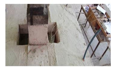
Figure 33: The Strain Gauge "red cable" is connected to the white cable of the Device for reading Strain results.
