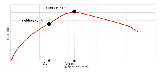
Figure 22: Indication for deducing Yielding point and Ultimate point from Load mid-span deflection curve.
