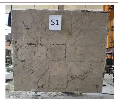
Figure 30: Failure Mechanism of the Post-tensioned Flat Slab during experimental tests. The appearance of cracks during increased load on the slab was numbered.
