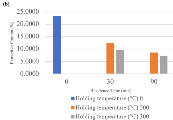
**Fig. 1.** (a) Effect of holding temperature on extractive content of raw and torrefied *Acacia mangium* biochar; (b) Effect of residence time on extractive content of raw and torrefied *Acacia mangium* biochar
