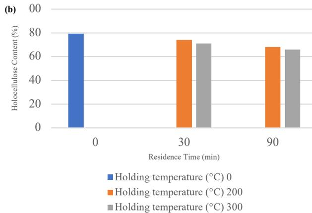
**Fig. 2.** (a) Effect of holding temperature on holocellulose content of raw and torrefied *Acacia mangium* biochar; (b) Effect of residence time on holocellulose content of raw and torrefied *Acacia mangium* biochar
