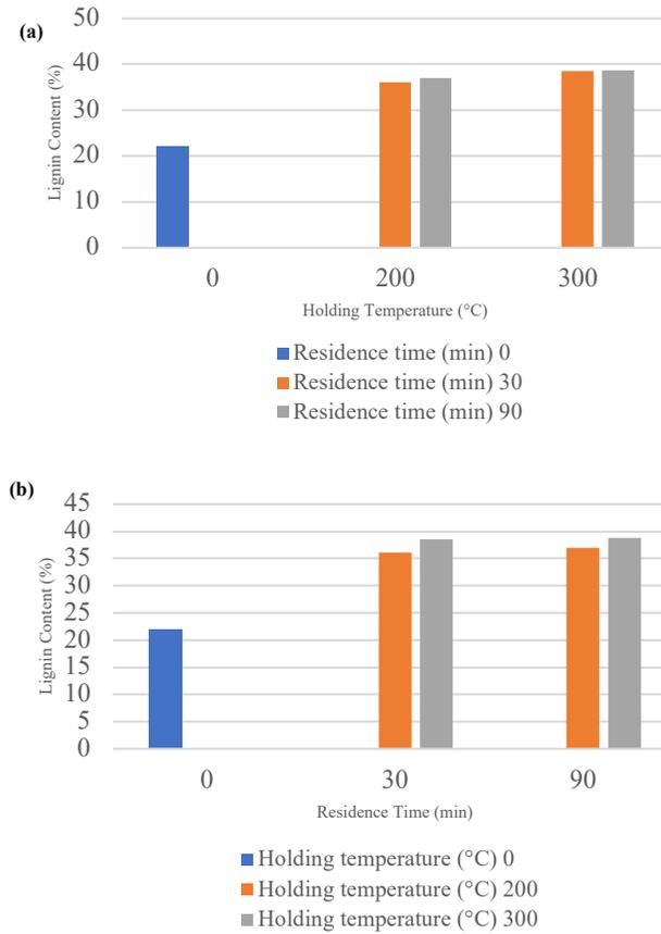
**Fig. 4.** (a) Effect of holding temperature on lignin content of raw and torrefied *Acacia mangium* biochar; (b) Effect of residence time on lignin content of raw and torrefied *Acacia mangium* biochar
