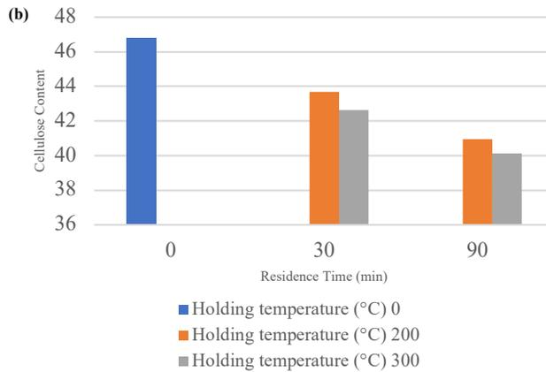
**Fig. 3.** (a) Effect of holding temperature on cellulose content of raw and torrefied *Acacia mangium* biochar; (b) Effect of residence time on cellulose content of raw and torrefied *Acacia mangium* biochar
