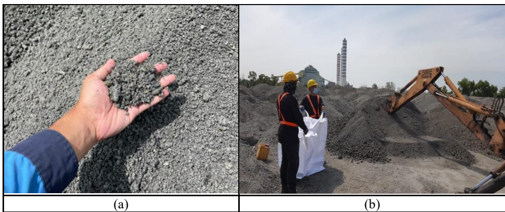
Fig. 1. Collection of CBA from Coal Ash Pond. (a) Condition of CBA during collection (b) Loading CBA into bulk bags for transportation.
