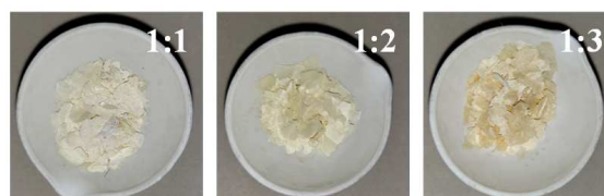
Fig. 8. Visual appearance of nitration result in various nitric acid : sulfuric acid ratio a) 1:1, b) 1:2, c) 1:3
