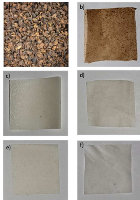
Fig. 2. Visual appearance a) Dried coffee pulp, b) Alkali Treated Coffee Pulp (ATCP), c) 2.5% Hydrogen peroxide bleaching (BL 2.5), d) 5% Hydrogen peroxide bleaching (BL 5), e) 7.5% Hydrogen peroxide bleaching (BL 7.5), f) 10% Hydrogen peroxide bleaching (BL 10)
